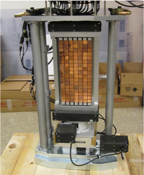
Double Focusing Pre-monochromator Copper Crystals
