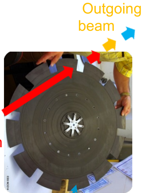
Chopper disk coated with neutron absorber
