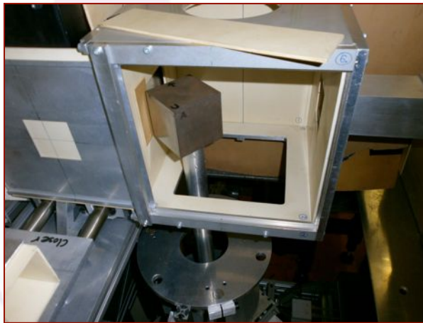
Neutron radiography (cold neutrons), ferritic steel cube at 45°.
