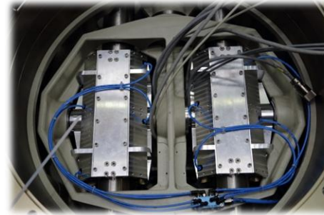
clamping system (A2 – sample position
