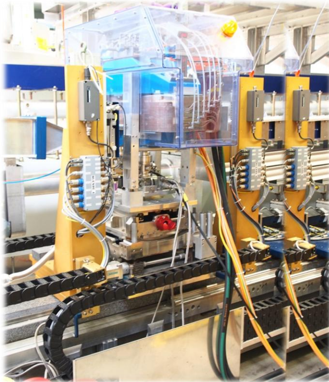
AMOR reflectometer sample table
