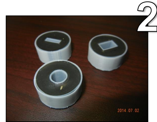
Molds With Enriched Boron Epoxy Mix
