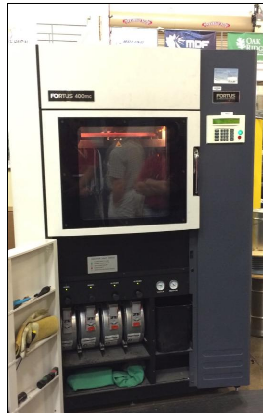
Stratasys Fortus 400, with lower door open, exposing its four filament cartridges
