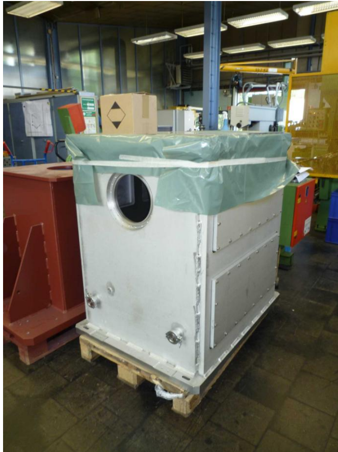
Fabrication of the vacuum chamber
