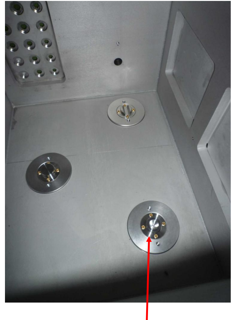
Three supports for the polarizer in the form of cones, spheres and flat support
