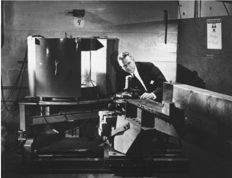
Walter Zinn at the neutron diffractometer on the CP-3 reactor
