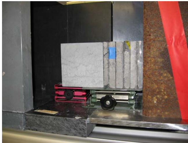
Sample with strong steel collimator (1m)
