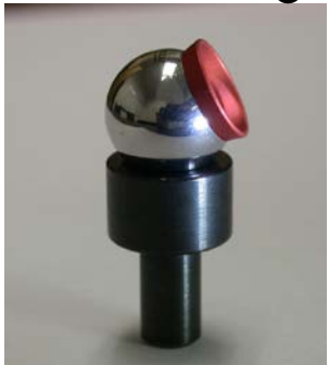
Nests for 0.5-inch reflector. Shank degrades repeatability.
