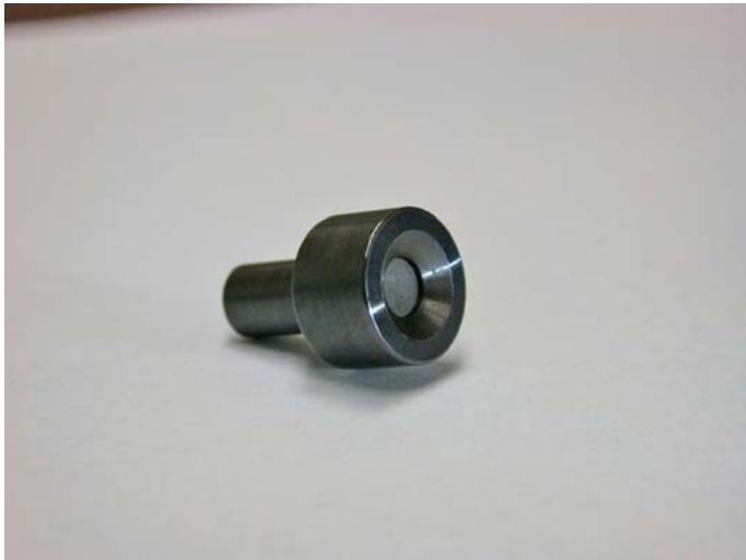
Nests for 0.5-inch reflector. Shank degrades repeatability.
