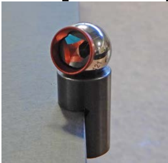
Nests for 0.5-inch reflector. Shank degrades repeatability.
